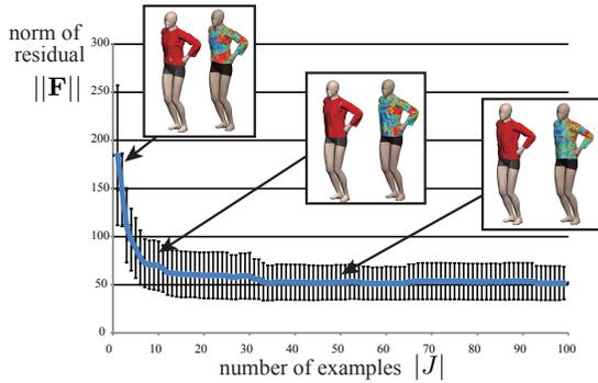
**Figure 12:** Convergence of residual norm during database construction. The blue line shows average of residual sampled over 400 random poses and the error bars show their standard deviations. The synthesized clothing and their residual distributions at the same pose are illustrated from the database with examples  $|J| = 2, 10, 50$ .
