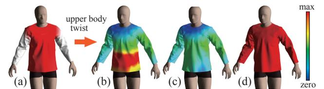
**Figure 5:** Distribution of  $\alpha$  for chest bone, showing global influence of this bone in the example pose (a). While there are unnatural wrinkles in the clothing deformation computed from local skinning weight only (b) with respect to upper body twist, our SOR method generates natural draping shape (c), which agree with ground truth equilibrium shape (d). The color bar here indicates the magnitude of  $\rho$  in Equation 7 that is difference from sensitivity analysis.
