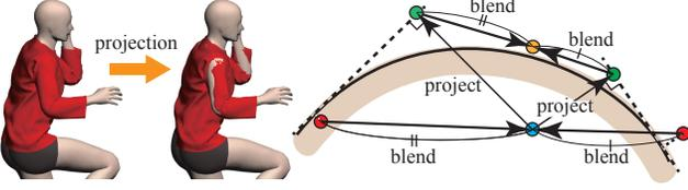
**Figure 8:** Our overall penetration resolution scheme. First, a clothing vertex is predicted for the input pose from its nearby example deformations (red points), and then they are blended into an intermediate vertex position  $\mathbf{y}^{in}$  (blue point). This is projected onto the body surface for each example  $\hat{\mathbf{y}}^J$  (green points). Finally, it is blended again to produce the final output position  $\bar{\mathbf{y}}^{in}$  (orange point).
