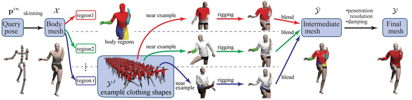
**Figure 3:** Overview of our clothing synthesis workflow. Given a query pose and a skinned body mesh, we firstly choose nearby clothing examples for each region. For each example, we deform the clothing mesh with the examples’ sensitivity-optimized rigging scheme (SOR). We then blend the deformations to synthesize an intermediate mesh. We then resolve penetrations and add dynamic effects and damping.
