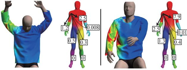
**Figure 6:** Distribution of differences in the sensitivity matrix over a clothing mesh. We compute the sensitivity matrix with respect to the rotation of the right shoulder joint. The numbers on the regions represent values of  $U_{g,m}^J$ .
